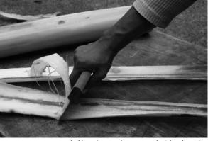
Banana stems are peeled into layers, then scraped with a broad, straightedged knife.
