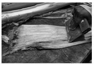
The extracted banana fiber is a lustrous raw material for papermaking.
